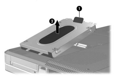
5. To insert the replacement hard drive, tilt the connector edge of the hard drive **1** downward, and then lower the hard drive into the hard drive bay until it is seated **2**.
